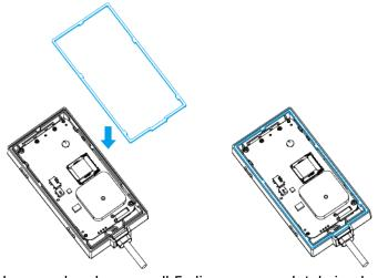
5. Press the upper case down and make sure all 5 clips are completely in place
