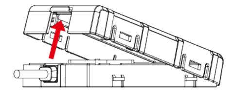
3. Insert SIM card into the slot and toggle the switch to ON
