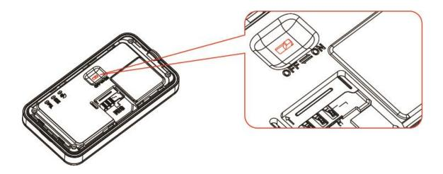
4. Close the SIM card cover and connect the device with the external power line which will be used to charge the terminal and built-in battery.
