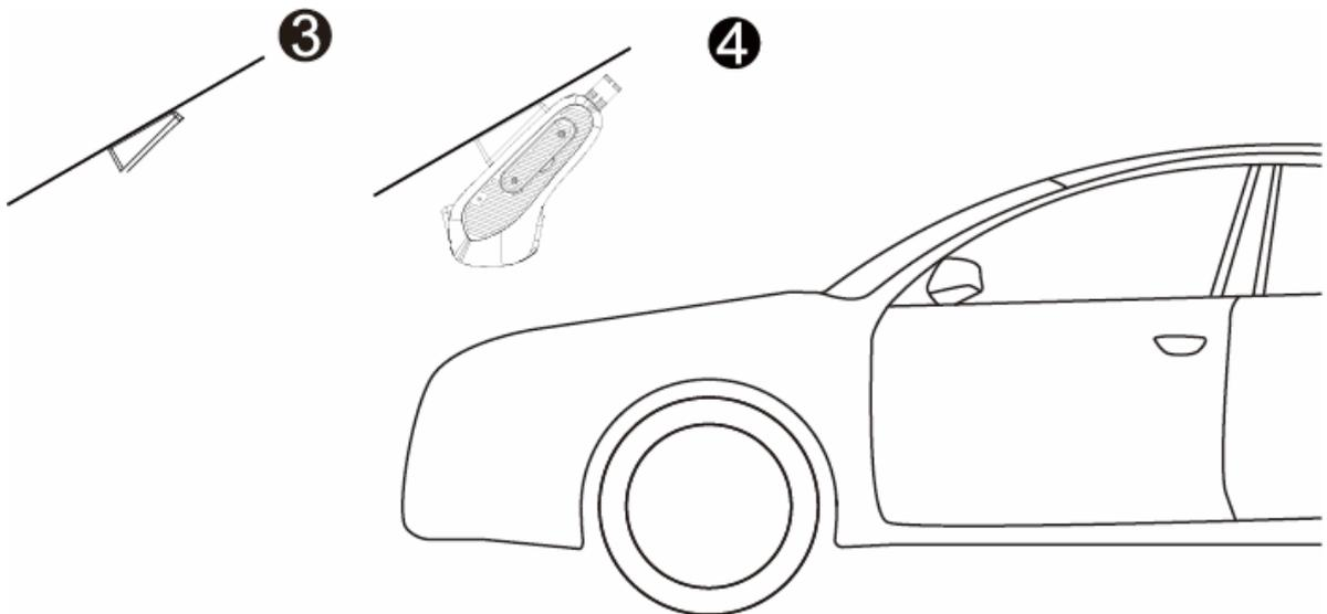
3. Select a proper installation position and wipe the position clean. Remove the protective film from the 3M tape of the mounting base and attach it to the position. Wait for 2 hours before proceeding to the next step. See **3** for reference.
