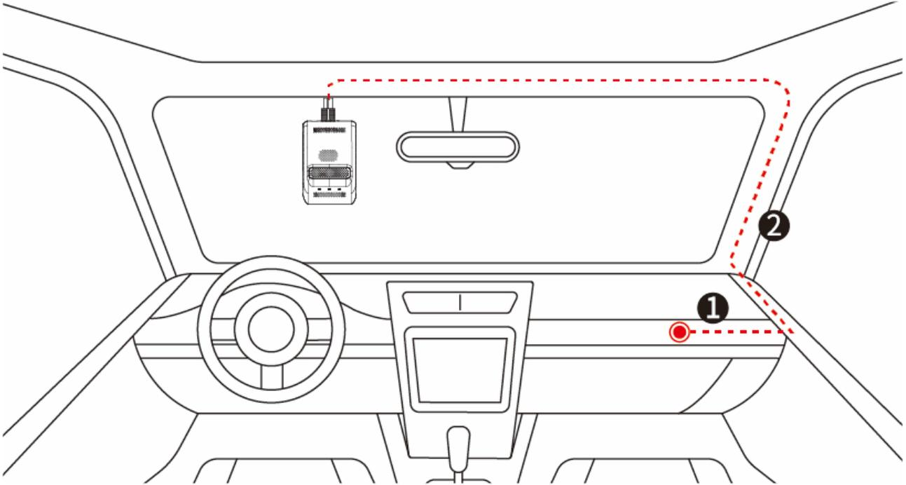
1. Connect the power cable of the device to B+, ACC, and GND of the fuse box on the vehicle. **1** is a reference position.
