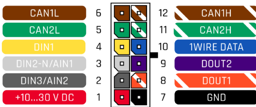
AIT20 2x6 socket pinout
