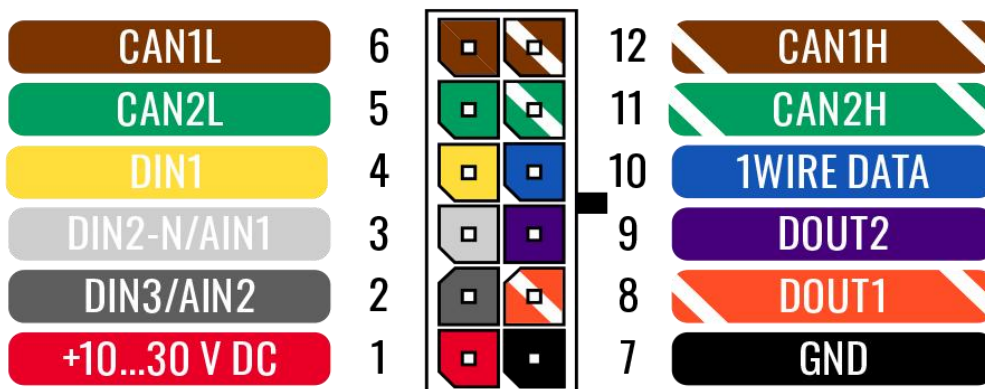
AIT200 2x6 socket pinout
